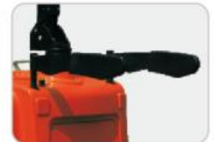
Protective arms are equipped on the both sides of driver's seats
