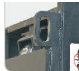
Lifting holes on the top of the mast
